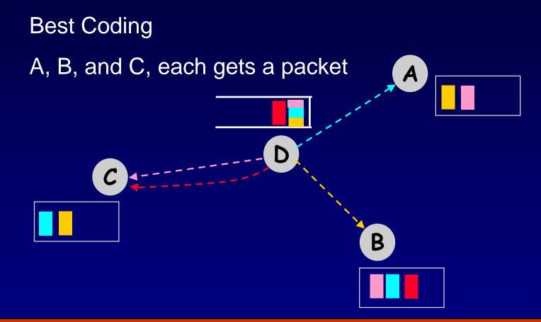
To XOR *n* packets, each next-hop should have the *n-1* packets encoded with the packet it wants
