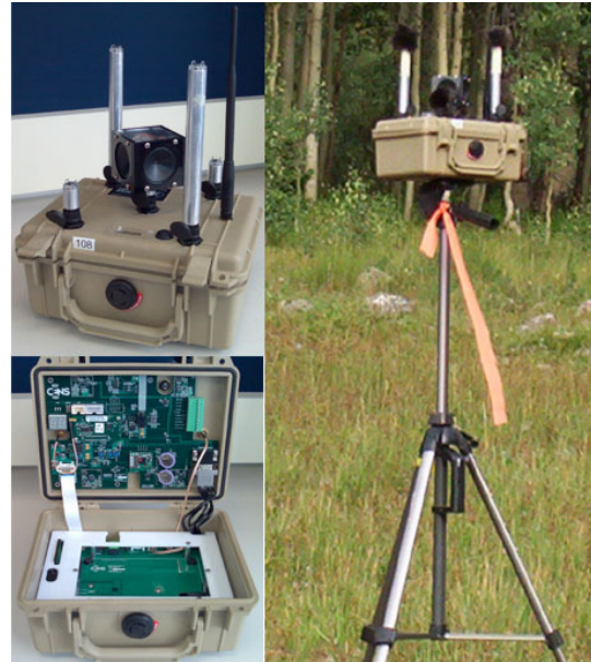
Figure 1. The packaged VoxNet node, shown in deployment at the Rocky Mountain Biological Laboratory, August 2007.
