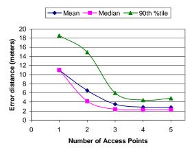
Figure 2: The effect of the number of access points on the error in the location estimate.
