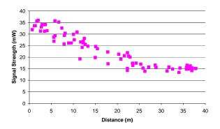
Figure 1: Empirically recorded profile of signal strength as a function of distance between transmitter and receiver.
