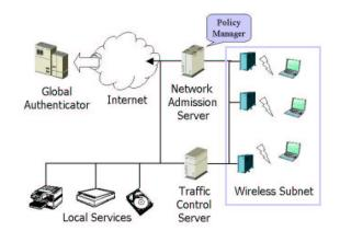
Figure 4: The architecture of the CHOICE public-area wireless network.
