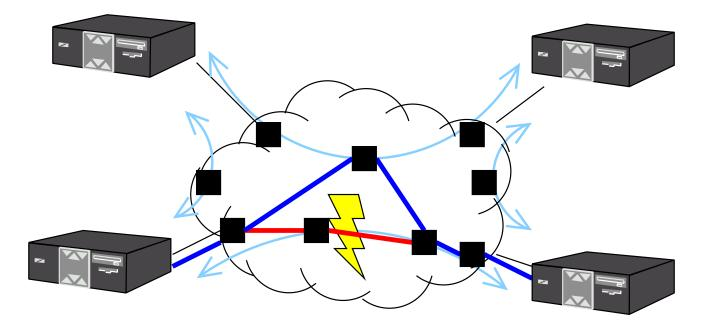
• Any-to-any communication transparently routing around failures
