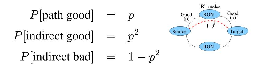
P[path good] = p  $P[\text{indirect good}] = p^2$   $P[\text{indirect bad}] = 1 - p^2$   $P[\text{indirect bad}] = 2 - p^2$
