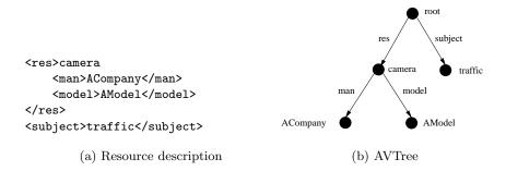
**Fig. 1.** Example of a very simple resource description and its corresponding AVTree. The resource is a camera, manufactured by ACompany and filming traffic
