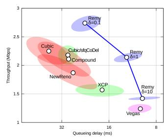
Figure 7: Verizon LTE downlink trace, n = 4. 1- $\sigma$  ellipses are shown. The RemyCCs define the efficient frontier. Senders alternated between exponentially-distributed file transfers (mean 100 kilobytes) and exponentially-distributed pause times (mean 0.5 s).
