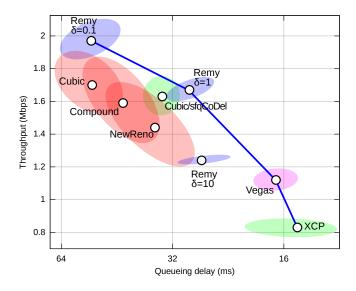
Figure 8: Verizon LTE downlink trace, n = 8. 1- $\sigma$  ellipses are shown. As the degree of multiplexing increases, the schemes move closer together in performance and router-assisted schemes begin to perform better. Two of the three RemyCCs are on the efficient frontier.
