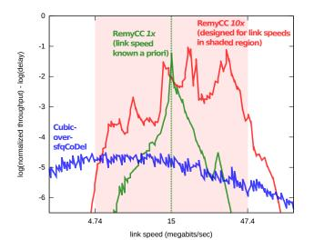
Figure 11: Performance of two end-to-end RemyCCs that were designed with different prior information about the network, compared with Cubic-over-sfqCoDel as the link speed varies. Despite running only at the sender, the RemyCCs each outperform Cubic-over-sfqCoDel over almost their entire design ranges. But when a RemyCC's assumptions aren't met, performance deteriorates.
