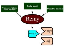
Figure 1: Remy designs congestion-control schemes automatically to achieve desired outcomes. The algorithms it produces may replace the congestion-control module of a TCP implementation, and fit into a network library or kernel module that implements congestion control (DCCP, SCTP, the congestion manager, application-layer transmission control libraries, ns-2 modules, etc.).
