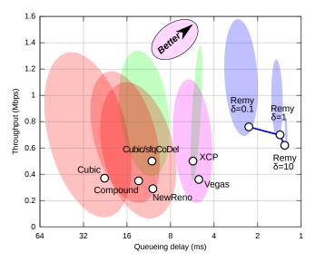
Figure 5: Results for the dumbbell topology with n = 12 senders, each alternating between flows whose length is drawn from the ICSI trace (Fig. 3) and exponentially-distributed off time (mean = 0.2 s). Because of the high variance of the sending distribution,  $\frac{1}{2}$ - $\sigma$  ellipses are down. The RemyCCs again mark the efficient frontier.
