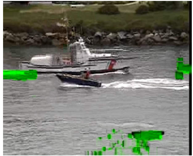
Figure 2: B-Frame #65 from “coastguard” stream showing propagation of errors. Y PSNR: 17.538345
