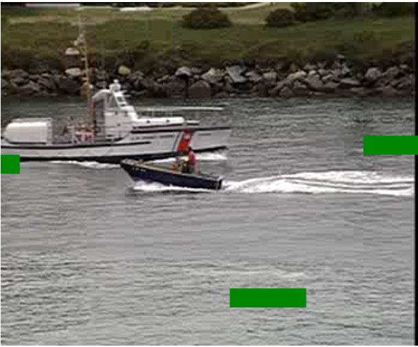
Figure 1: I-Frame #48 from the “coastguard” stream with packet loss. Y PSNR: 21.995697
