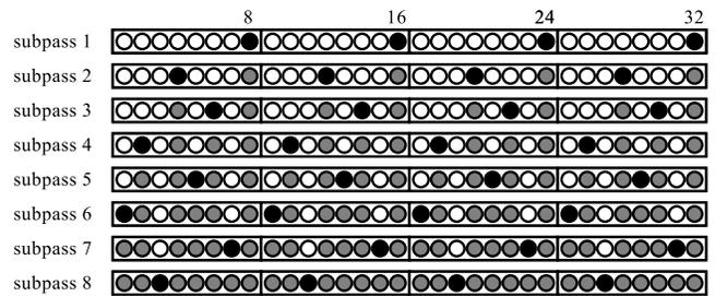
**Figure 4: Puncturing schedule.** In each subpass, the sender transmits symbols for spine values marked by dark circles; shaded circles represent spine values that have already been sent in a previous subpass.
