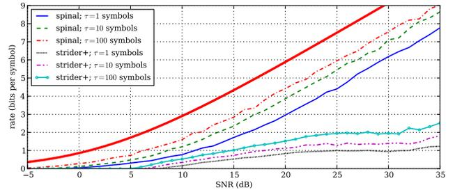
**Figure 11: Performance of the AWGN decoders on the Rayleigh simulation. This experiment examines the decoders' resilience to varying or inaccurate channel information.**
