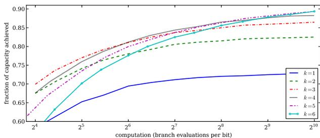
**Figure 12: How compute budget per bit ( $B2^k/k$ ) affects performance in the SNR range 2-24 dB, for different  $k$ . A choice of  $k = 4$  yields codes that perform well over the entire range of budgets. This graph also shows that  $B = 256$  is a good choice.**
