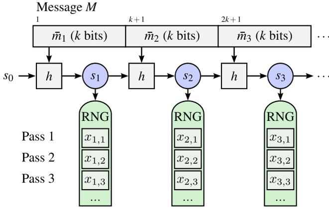
**Figure 1: Encoding process.** Start with a hash function,  $h$ . Compute spine values  $s_i = h(s_{i-1}, \bar{m}_i)$ . Seed RNG with  $s_i$ . For pass  $\ell$ , map  $c$  bits from RNG to symbol  $x_{i,\ell}$ .
