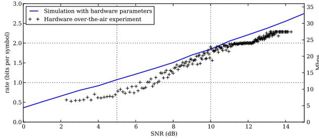
**Figure 9: Rates achieved by the hardware over-the-air experiment, compared to a software simulation with similar parameters. Throughput (right axis) shows equivalent link rate for a 20 MHz 802.11a/g channel.**
