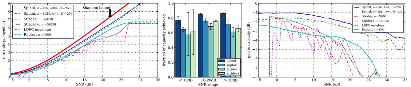
**Figure 6: Rates achieved by spinal code with  $k = 4$ ,  $B = 256$ ,  $d = 1$ , and the other codes (Strider+ is Strider with our puncturing enhancement). Experiments at each SNR average Raptor performance over 100-300 kbits of data, Strider over 5-20 Mbits, LDPC over 2 Mbits, and spinal codes over 0.6 to 3 Mbits.**
