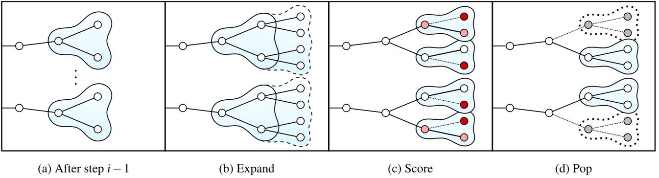
**Figure 3: Sequential decoding process using the bubble decoder with  $B = 2$ ,  $d = 2$ ,  $k = 1$ .** (a) At the beginning of step  $i$ , the partial trees have depth  $d - 1$ . (b) Grow them out to depth  $d$ . (c) Propagate the smallest path costs back through the tree. (d) Select the  $B$  best children, pruning the rest. Advance to the next step and repeat.
