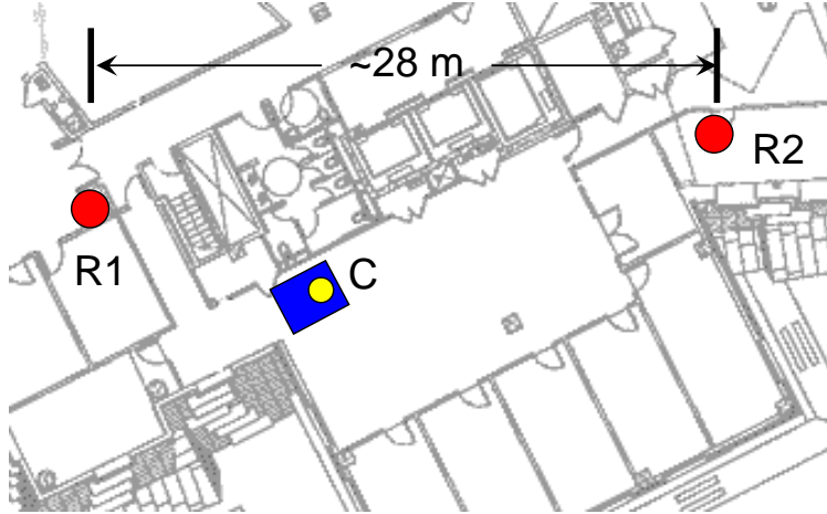
Figure 3-8: Setup for the HIVAR experiments. R1 and R2 are stationary receivers. C is a laptop transmitter client that was carried by a walking person who covered a 1.5 \text{ m} \times 2 \text{ m} area during the experiments.
