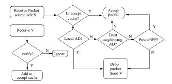
Figure 3: Process for verifying a packet's source address.
